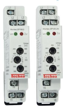
These relays monitor overvoltage and undervoltage in 3 Phase AC systems (they do not monitor phase sequence and phase failure). The Montec-3PVM-2 draws its supply from 3 live phases, which means that the relay remains functional even if one phase is lost. The Montec-3PVM-2N draws its supply from L1, L2, L3 and N, so the relay also monitors loss of the neutral.
